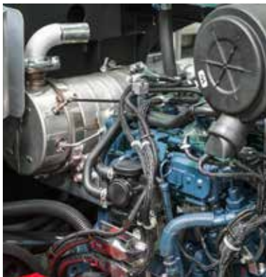
Tier 4/Stage V ready engine with built-in diesel particulate filter and catalyst
